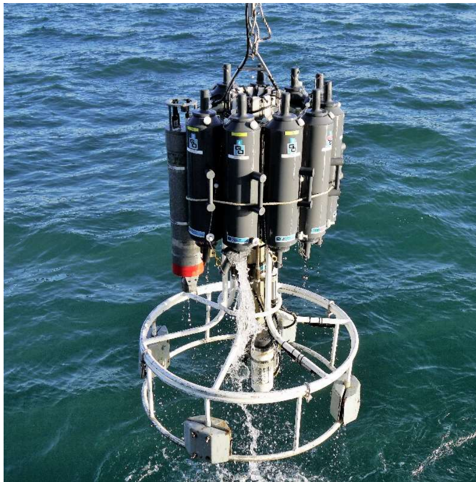
Figure 2.3: Rosette sampler used during the 13-hour cycles. Attached on the rosette are 5l Niskin bottles, a SBE09 CTD system with OBS and a LISST 100.
